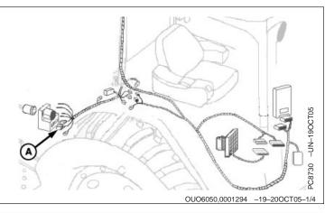
NOTE: FOR TRACTORS EQUIPPED WITH A TECU: Implement connector can not be used as the source of the 2-pin power on machines equipped with a TECU. Kits PF80873 or PF80874 provide a connection point for 2-pin power.
